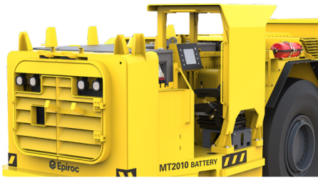
Operators compartment with a side-seated canopy for bi-directional operations.
