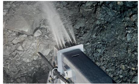
The water sprinkler system provides efficient dust control.
