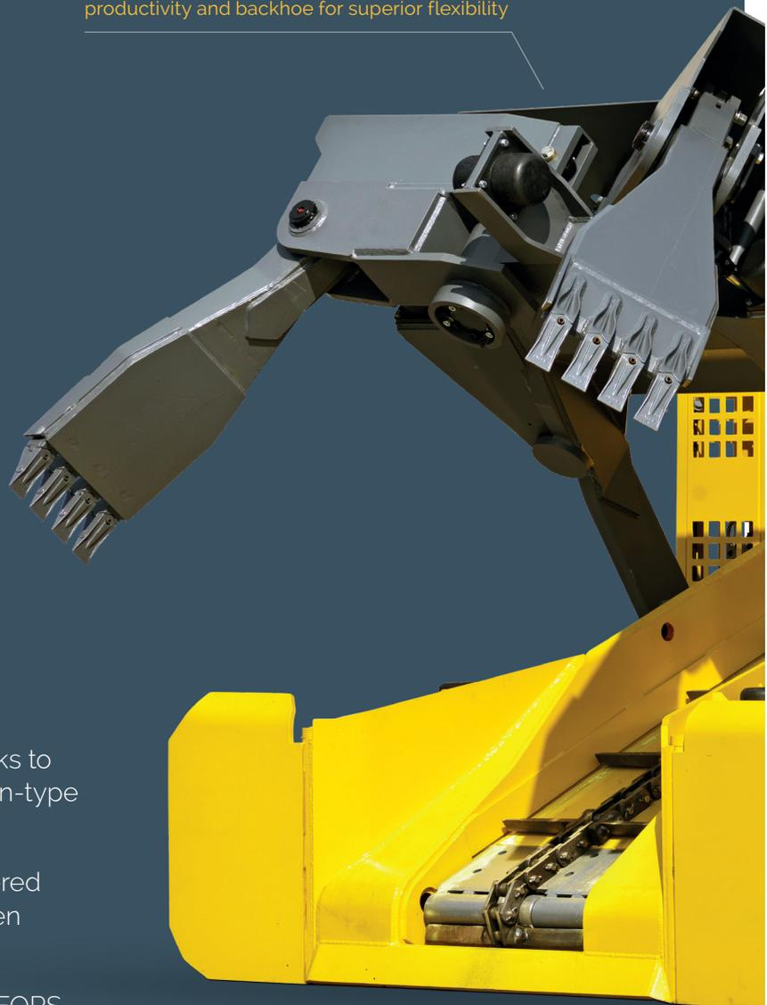
Strong, centrally mounted chain with wing-shaped flights allows stacked material to pass
