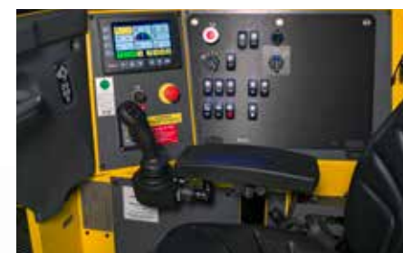
Focus on your task and be productive with the controls you have in close reach on the joystick.
