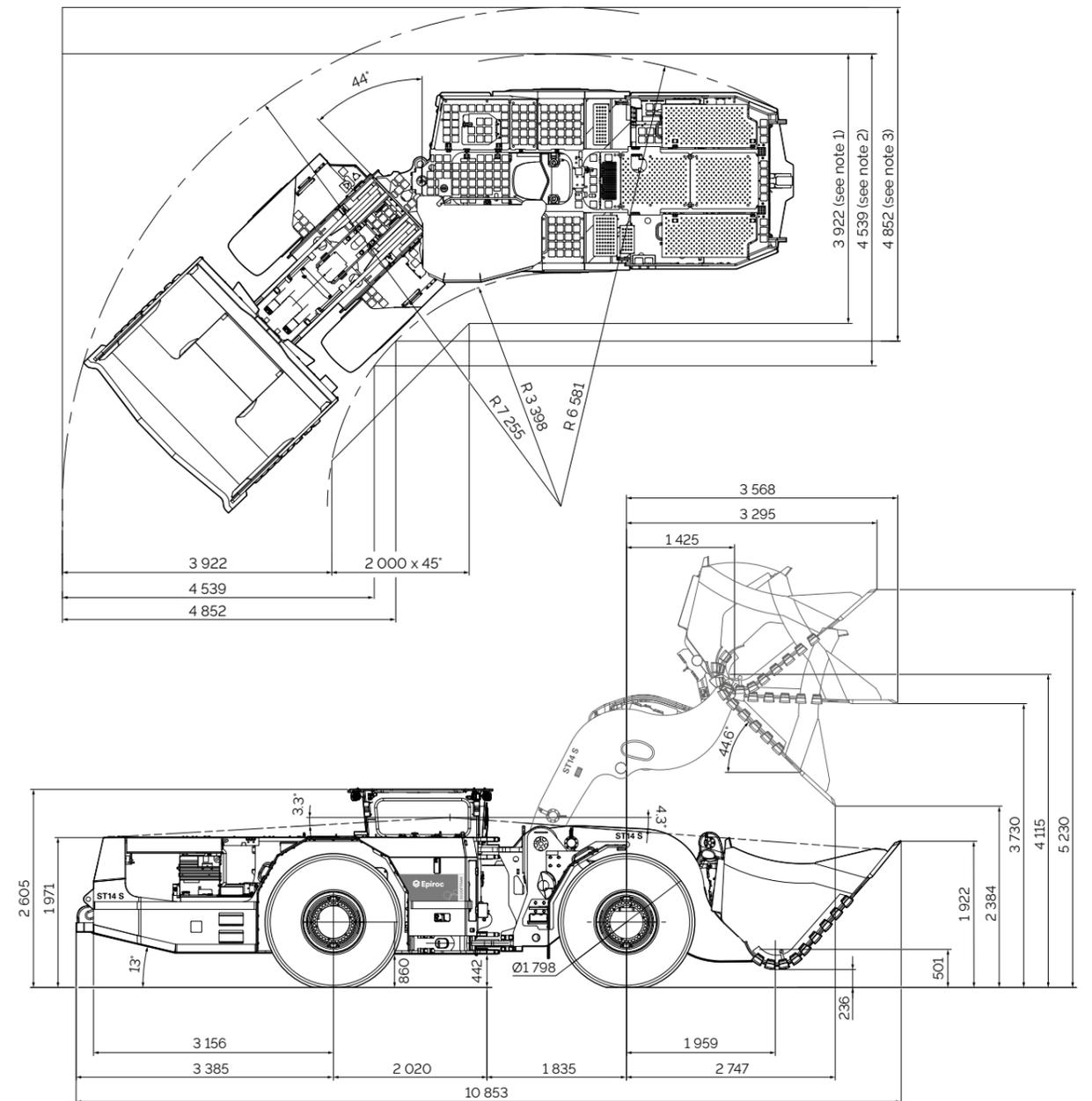
All dimensions are shown in millimeters (mm). Dimensions and calculations shown are based on standard vehicle configuration with 27 mm tire deflection, unloaded.
