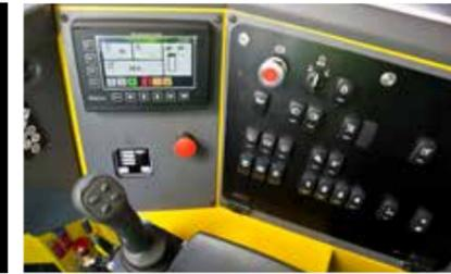
Scooptram ST14 S has a smart control system featuring traction control, speed limiter, over speed protection and automatic ride control.
