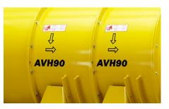
To maintain extra-high pressure, up to five units of any diameter and motor size can be connected in series at a single fan station
