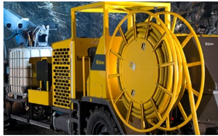
The integrated dosing system for liquid additives guarantees continuous flow through the interaction of flowmeter, frequency converter and controller
