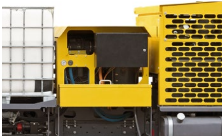
75 kW onboard compressor for optimal delivery of sprayed concrete
