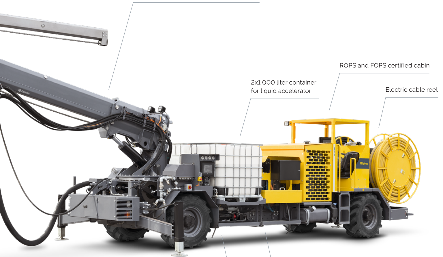
Sturdy carrier with permanent electronic 4-wheel drive with ASS and TCS
