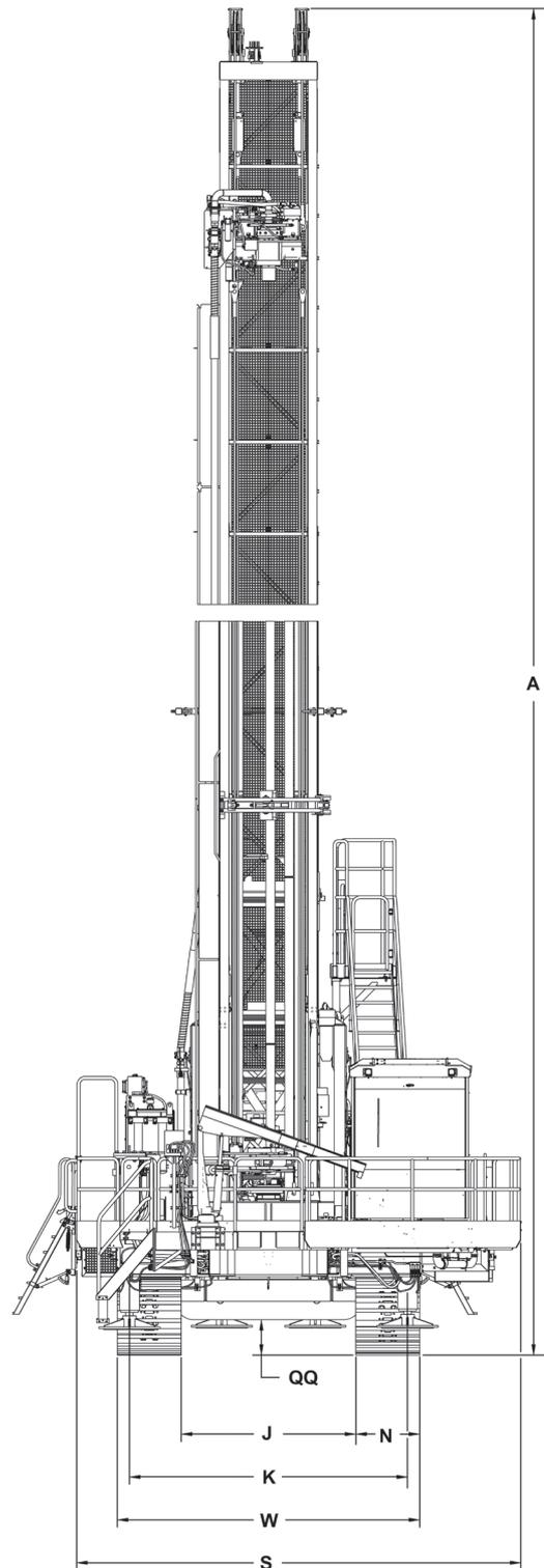
\*Approximate shipping dimensions for crated Pit Viper 271 XC (actual dimensions will vary based on rig configuration).
