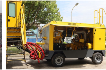
Connection Kits: Tailored to the suit hydraulic system of drill with common connection to Motivator unit allowing the Motivator to be compatible with mixed fleet operations.
