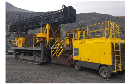
RRC: The Radio Remote Control (RRC) option lets the operator control propelling functions from a safe, remote location. Basic machine setup functions available with rescue function option.
