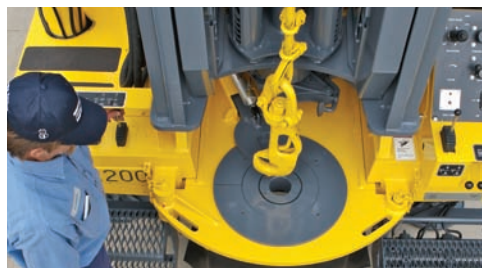
Head Retracted - Hoist Line on Center
