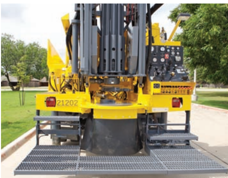
Work Area with Platforms
