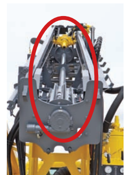
Head Ready to Load Pipe
