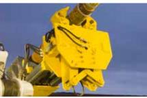
The Driller has complete control over the Predator drill pipe to top drive connection process by clamping and extending the drill pipe to the top drive and threading into the pipe for a secure connection before bringing the drill pipe in through the drill floor.
