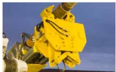
The Driller has complete control over the Predator drill pipe to top drive connection process by clamping and extending the drill pipe to the top drive and threading into the pipe for a secure connection before bringing the drill pipe in through the drill floor.
