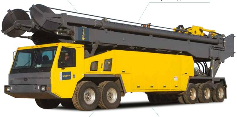
The Predator carrier is hydrostatically driven via a hydraulic motor powered by the deck engine diesel hydraulic system, eliminating the need for a dedicated carrier engine.
