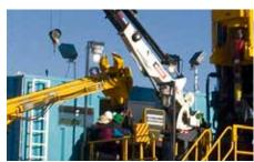
The Predator Pipe Skate features hands free pipe handling from the pipe racks all the way to the pipe connection via wireless remote controller.
