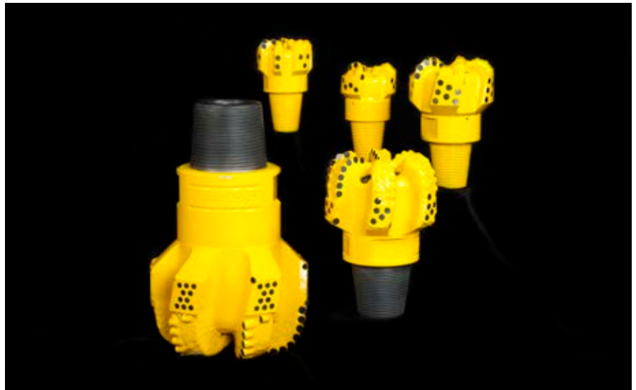
PDC bits, such as the Atlas Copco "Dirt Digger" line, feature polycrystalline diamond compact inserts on the cutting faces. The flat parabolic design of these bits offers maximum protection while drilling in non-homogenous and unconsolidated formations.
