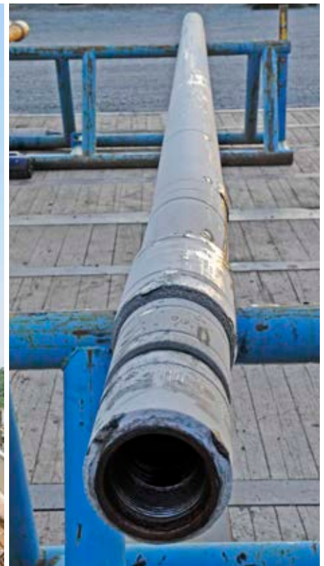
Left: This job was performed with an Atlas Copco RD20 using mud to drill directionally. It called for a large shaker box (on the right) and two large mud pumps to deliver clean mud to drive the directional mud motor. Right: This air motor used for directional drilling looks the same as a mud motor. This particular motor was used in a job requiring a bend of 1.25 degrees.
