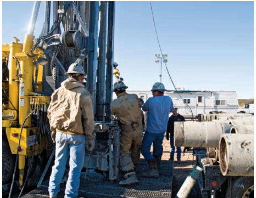
The tophead of the RD20 XC, which has bails and a hydraulically activated elevator rated to 120,000 pounds (54 metric tonnes), is specifically designed for bottleneck pipe handling.
