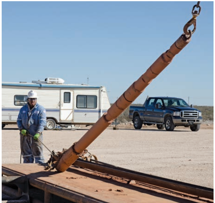
From the bit to the drill pipe multiple crossover connections drop the size from 6 1/2 to 4 1/2 inches. A shock-sub in this section absorbs half the bounce from the bit to the rotary head.
