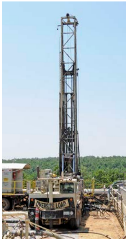
Left: This job was performed with an Atlas Copco RD20 using mud to drill directionally. It called for a large shaker box (on the right) and two large mud pumps to deliver clean mud to drive the directional mud motor. Right: This air motor used for directional drilling looks the same as a mud motor. This particular motor was used in a job requiring a bend of 1.25 degrees.
