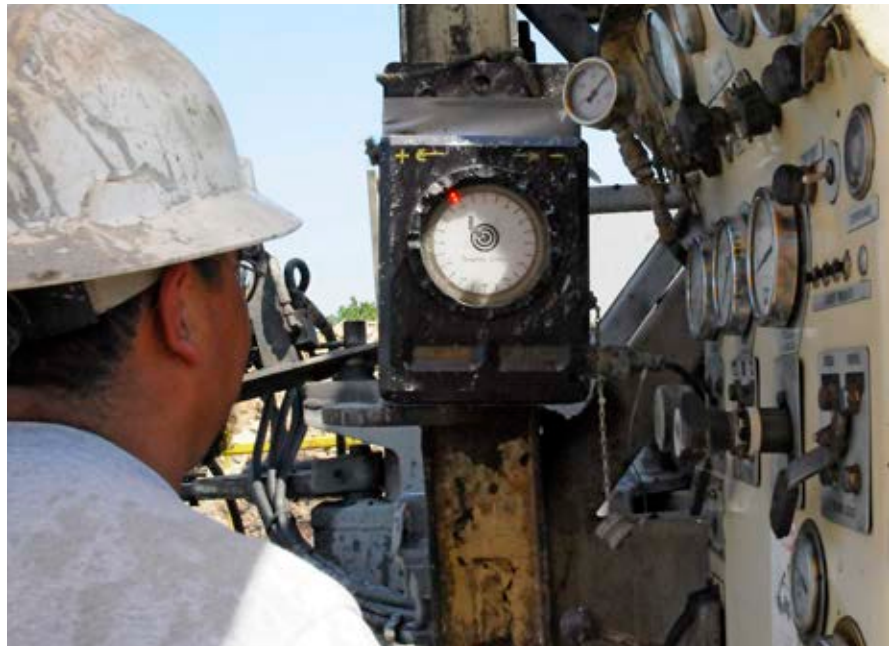
The driller is watching the angle that the mud motor is taking, indicated by the light on the dial. This particular job is drilling 240 degrees southwest.
