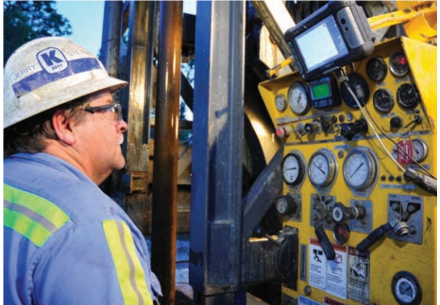
The EDGE drill monitoring system "reads" drill string vibration, showing performance data on a display at the driller's station. This real-time information allows the driller to constantly monitor drilling conditions in the hole and make adjustments as needed.
