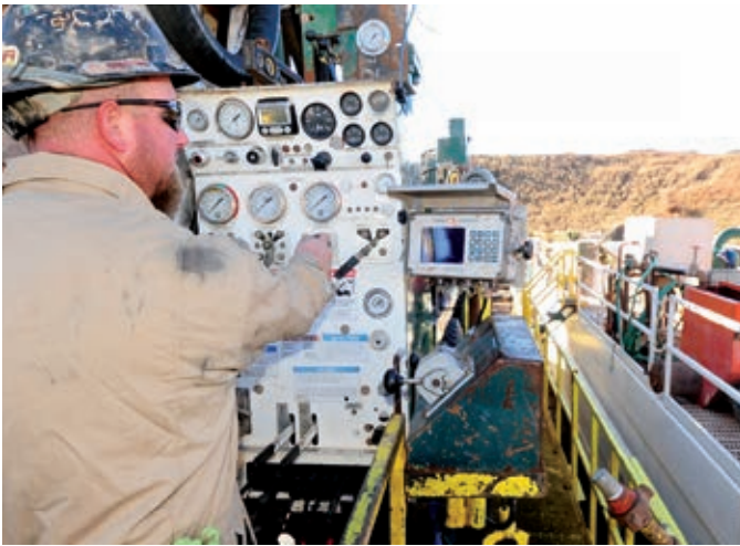
The RD20's workspace design offers a driller a good vision of mud system and rig operation from the driller station.
