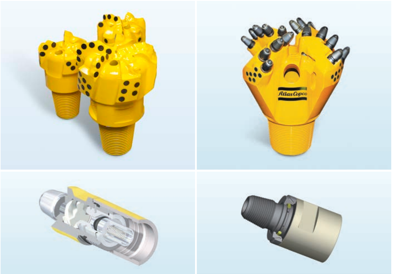
Top left: These “Dirt Digger” PDC bits feature polycrystalline diamond compact inserts on the bit’s blades to cut and ream a hole by shearing material away. Top right: The cutters on a Klaw bit are placed at specific locations to attack angles for maximum formation removal. Bottom left: The hydrocyclone keeps fluids from reaching the hammer. Bottom right: Jet subs prevent over-pressuring of the hammer in certain applications.
