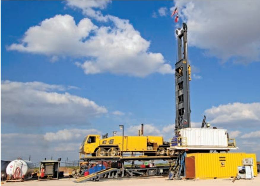
An Atlas Copco Predator oil and gas drilling system in operation shown positioned on its substructure. Predator is the largest of the Atlas Copco line of carrier-mounted deephole drill rigs. Its 220,000 pounds (90,800 kg) of hookload allows drillers to bore vertical, directional and horizontal wells to depths of 8,000 feet (2,400 m) in today's global oil, CBM and natural gas basins.
