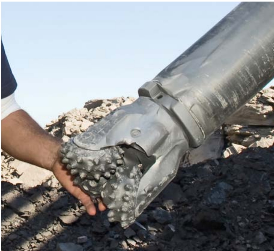
The downward force necessary for optimum bit performance depends on the size of the tooling and the increasing weight of the drill string as the hole advances.
