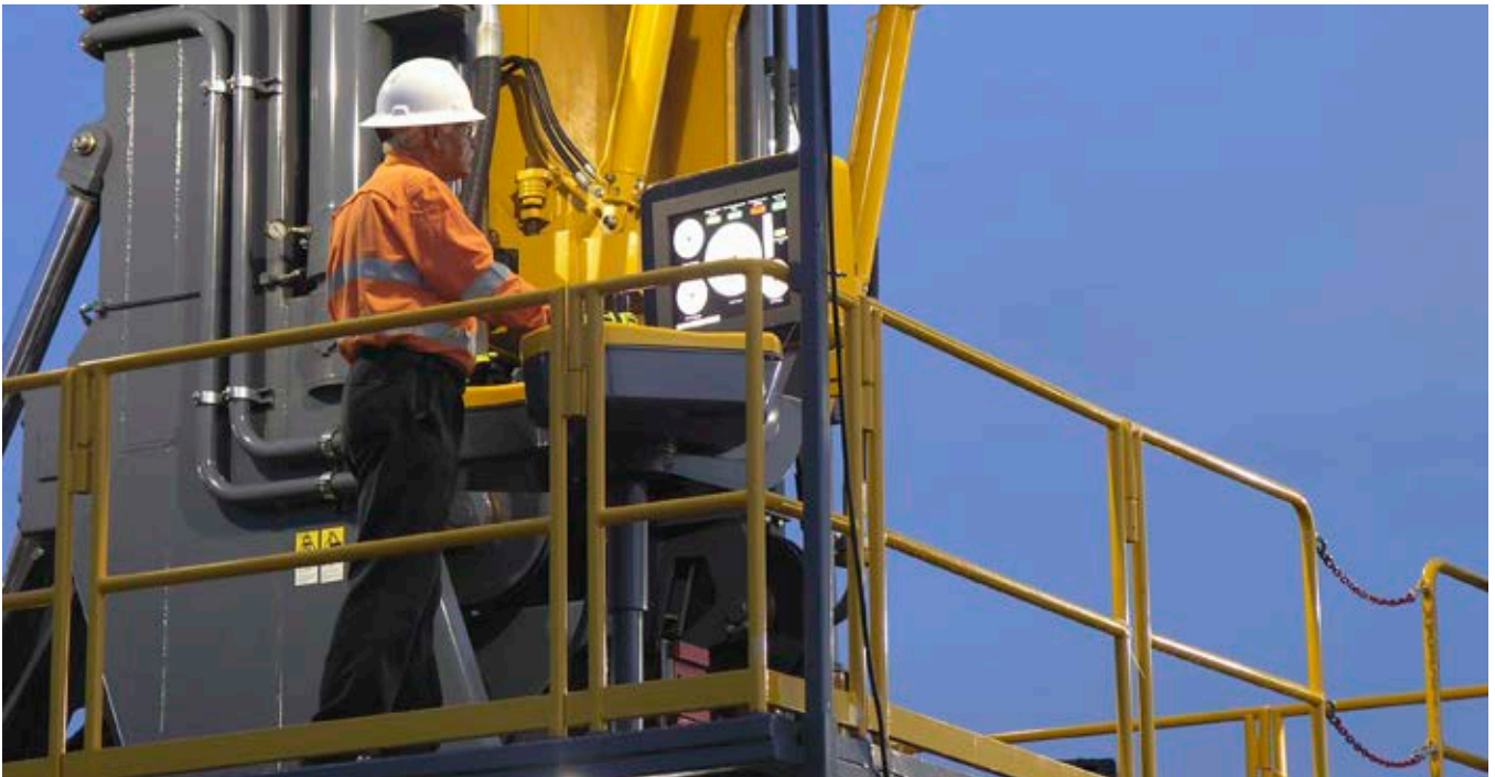
The Predator Drilling System has a tilt-out top drive that rotates out to receive pipe from its pipe skate. It achieves truly hands-free pipe handling.
