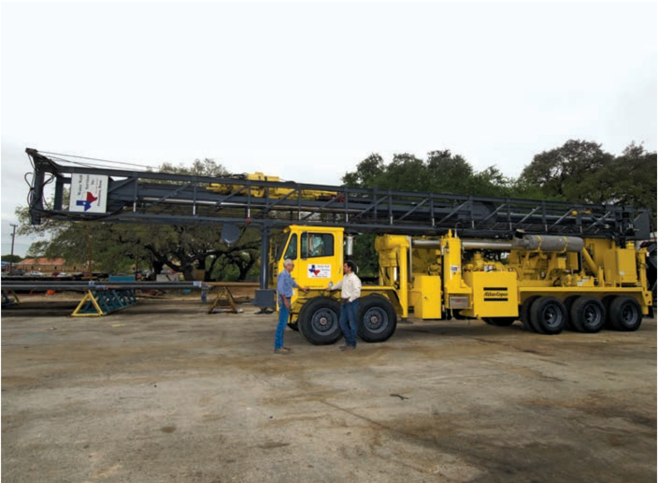
Richard Bartosh, drilling superintendent for Water Well Services Inc., discusses with Mike Epley of Venture Drilling Supply (at right) how the RD20 III XC performed drilling a 450-foot, 17.5-inch diameter well on the Carizzo-Wilcox aquifer 30 miles south of San Antonio.
