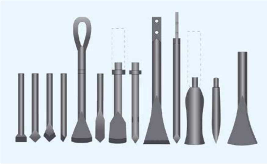
Broad and side views of seven styles of spring pole bits. The first two pairs of images on the left are two rock bits for quarrying. The remainder are a range of bit shapes created for various ground conditions by drilling pioneers such as David and Joseph Ruffner, Billy Morris and Levi Disbrow.
