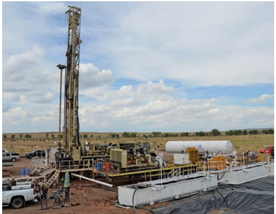
The site layout included both mud and air drilling options. Shown here are the mud boxes between the compressor trailer and pits.
