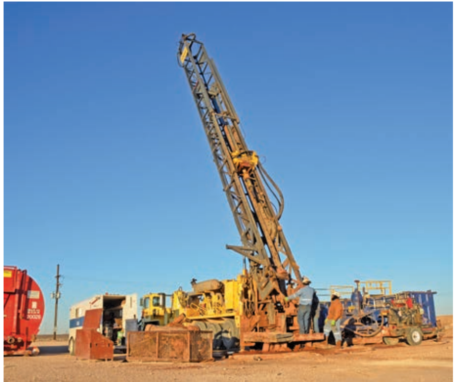
The RD20 drill rig's quicker set up time and far fewer trailer-loads of drilling and ancillary equipment compared to conventional oil and gas rigs result in increased productivity and greater economy.
