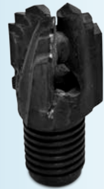
The sharp edges on the carbide blades of a drag bit shear formation material from the bottom of the hole.
