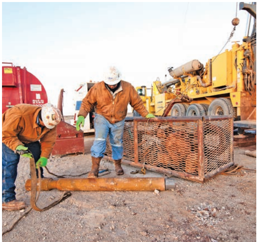
Packing up gear and tooling is quick with the cage and winch. The cage easily loads on a flatbed to move to the next site.
