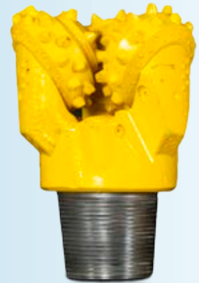
A tricone bit has three roller cones on one bit body, each placed so that its buttons complement those of the cones on either side of it. It can be used for rotary air and rotary fluid drilling methods.
